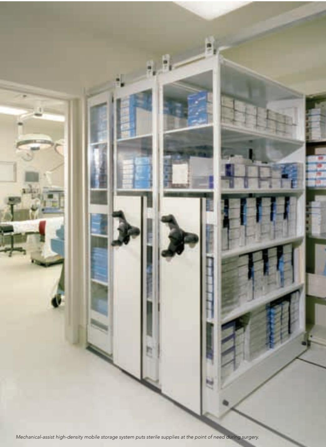
Mechanical-assist high-density mobile storage system puts sterile supplies at the point of need during surgery.
